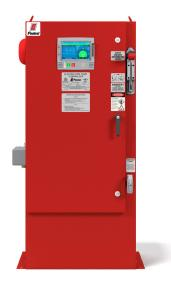
Description-Firetrol® FTA1300 Wye-Delta, Open Transition Starting Fire Pump Controllers are used with delta-wound squirrel cage motors. FTA1300 controllers are of the open circuit transition type in which the motor circuit is opened during the transition from start to run. The controller monitors, displays and records fire pump system information.
