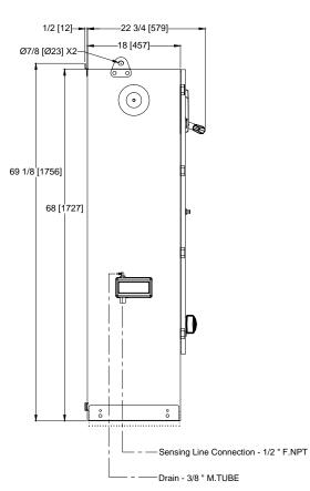
NOTE: DRAIN CONNECTION MUST BE PIPED TO WASTE DRAIN. FAILURE TO CONNECT TO A FLOOR DRAIN WILL RESULT IN UNSAFE CONDITIONS OF STANDING WATER AROUND CONTROLLER.
