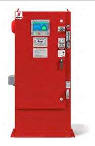
Description-Firetrol® FTA1350 Wye-Delta, Closed Transition Starting Fire Pump Controllers are used with delta-wound squirrel cage motors. FTA1350 controllers are of the closed circuit transition type in which the motor circuit remains closed during the transition from start to run. The controller monitors, displays and records fire pump system information.
