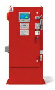
Description—Firetrol® FTA1350 Wye-Delta, Closed Transition Starting Fire Pump Controllers are used with delta-wound squirrel cage motors. FTA1350 controllers are of the closed circuit transition type in which the motor circuit remains closed during the transition from start to run. The controller monitors, displays and records fire pump system information.
