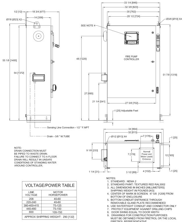
10. SEISMIC MOUNTING TO BE RIGID WALL AND BASE ONLY
