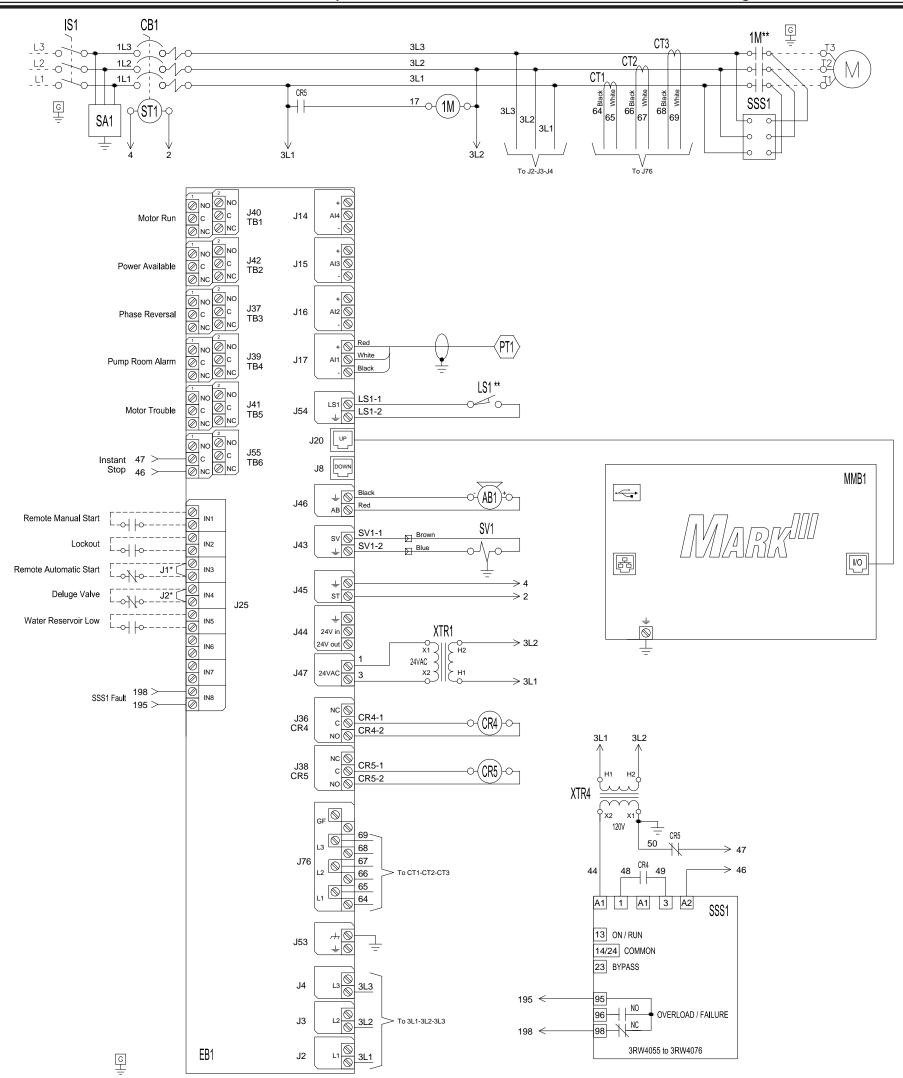
\* Remove jumper to use this feature \*\* Contact closes when emergency start is in "ON" position
