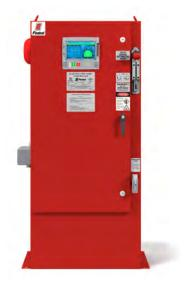
**Description** – Firetrol<sup>®</sup> FTA1000 Full Voltage Fire Pump Controllers are intended for use with electric motor driven fire pumps where the capacity of the power source permits full voltage starting. Full voltage is applied to the motor as soon as the controller is actuated. The controller monitors, displays and records fire pump system information.
