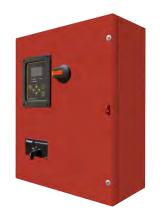
**Description**—Firetrol® FTA550E JockeyxG Pump Controllers are intended for use with fire pump systems. They are used for pressure maintenance in fire pump installations to prevent unnecessary operation of the main fire pump.
