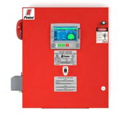
**Description** – Firetrol<sup>®</sup> combined automatic and manual MARK<sup>III</sup> based diesel engine fire pump controllers are intended for starting and monitoring fire pump diesel engines. They are suitable for use with both mechanical and electronic type engines. The controller is available for 12 or 24 volt negative ground systems, using lead acid or Nickel-Cadmium batteries. The controller monitors, displays and records fire pump system information.
