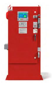
**Description** – Firetrol\* FTA1000 Full Voltage Fire Pump Controllers are intended for use with electric motor driven fire pumps where the capacity of the power source permits full voltage starting. Full voltage is applied to the motor as soon as the controller is actuated. The controller monitors, displays and records fire pump system information.
