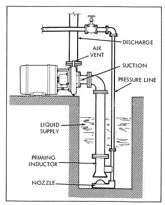
FIGURE 8. INDUCTOR PRIMING
