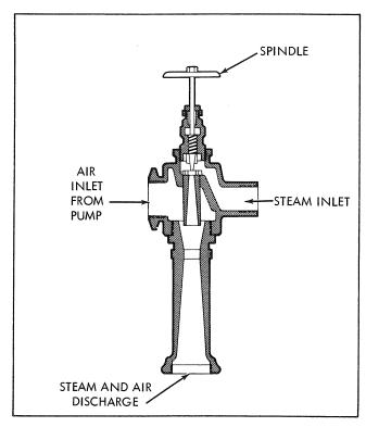
FIGURE 6. EJECTOR CUTAWAY
