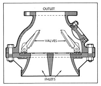
FIGURE 4. FOOT VALVE CUTAWAY
