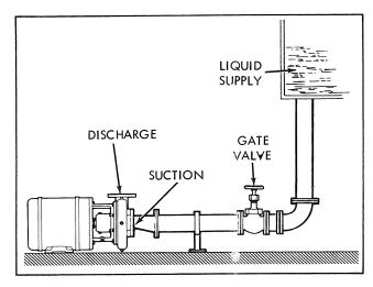
FIGURE 2. FLOODED SUCTION PRIMING
