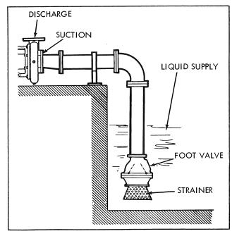
FIGURE 3. PRIMING WITH A FOOT VALVE
