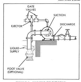
FIGURE 5. PRIMING BY EJECTOR
